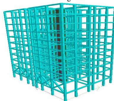
Figure 4.6 Property of G+10 soft storey structure without bracings
